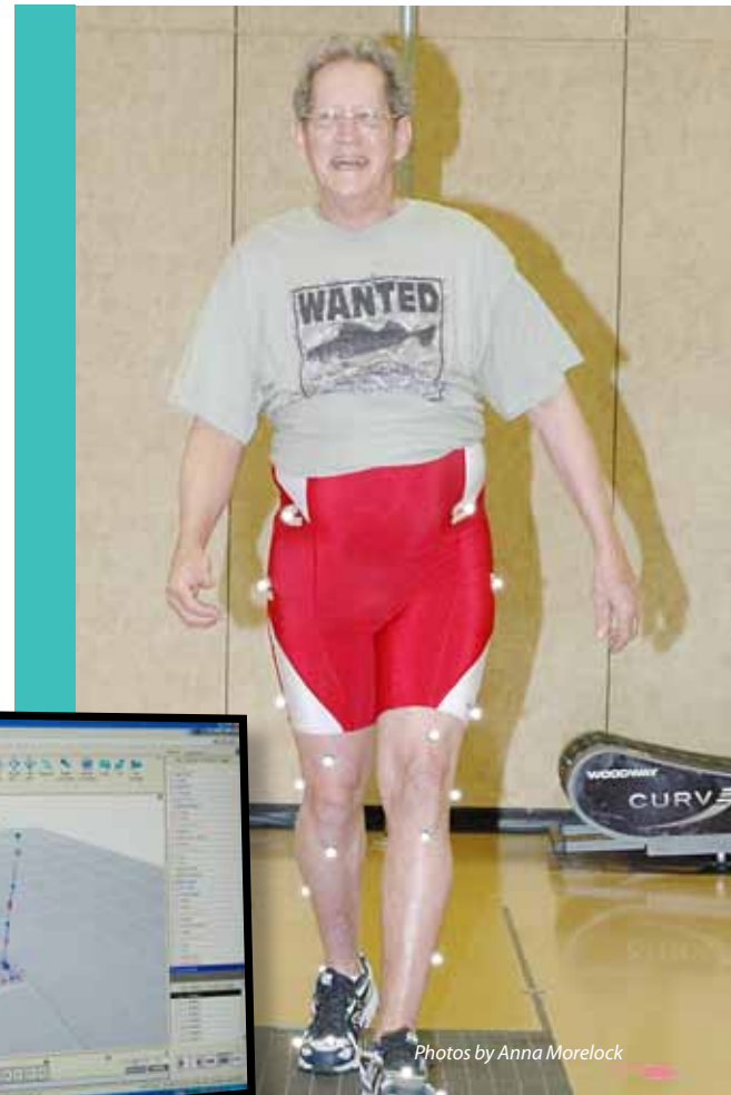
Army Veteran Kim Vanderloo participates in biomechanics testing at the University of Nebraska at Omaha Biomechanics Core Facility. The reflective markers on Vanderloo's feet and legs help lab technicians create a 3D model of Vanderloo on the computer (inset) to measure his gait. Vanderloo was completing the testing after having vascular surgery on his legs as a part of a research study through NWHCS.
